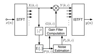
Figure 2.2: STFT-based stationary noise suppressor (from the Audio Signal Processing and Virtual Acoustics books[5]).
