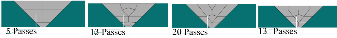
(a) Welding passes profiles for the four cases used in the study
