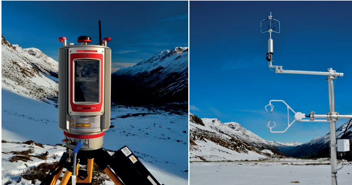
Fig 1.1 Terrestrial laser scanner (left) and an eddy-covariance tower (right) at the Gletschboden area, Davos, Switzerland
