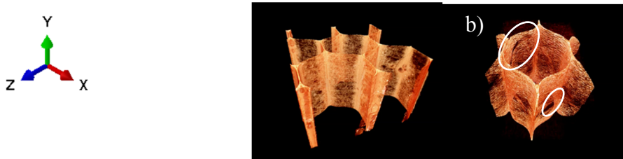
Fig. 6 : (a) 3D view of honeycomb cell before failure. (b) 3D view of honeycomb cell after failure.
