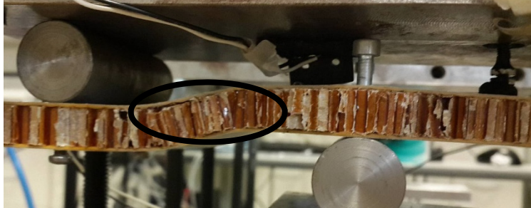
Fig. 5: Core shear failure in honeycomb sandwich at f=2\text{Hz} and 0.30\text{ MPa} .
