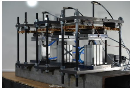
Fig. 2: Developed four-point test machine.
