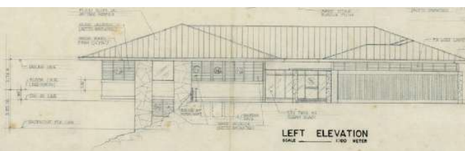
Leandro Locsin_ Residence John Tuason Jr(1960)_Quezon City Elévation montrant le porte-à-faux Source: Archives du bureau, photo Neal Oshima
