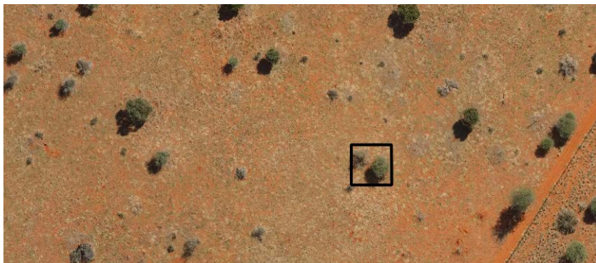
Figure 6.3: Size of a Sentinel-2 pixel, 10x10 meters. The background image is zone 1 in 2015
