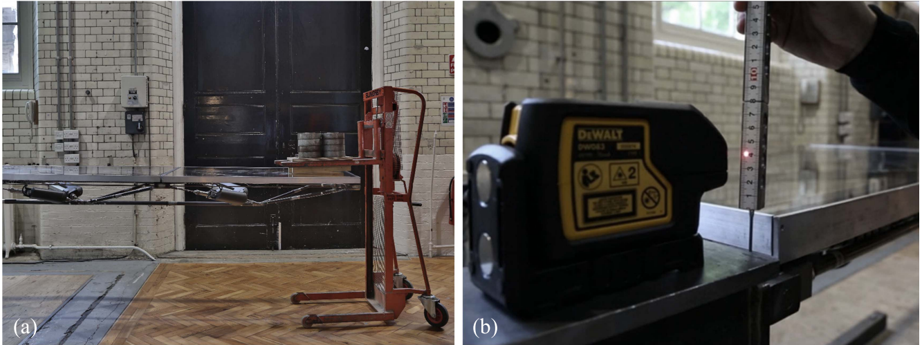
Figure 18. (a) Load test; (b) node displacement measurement.
