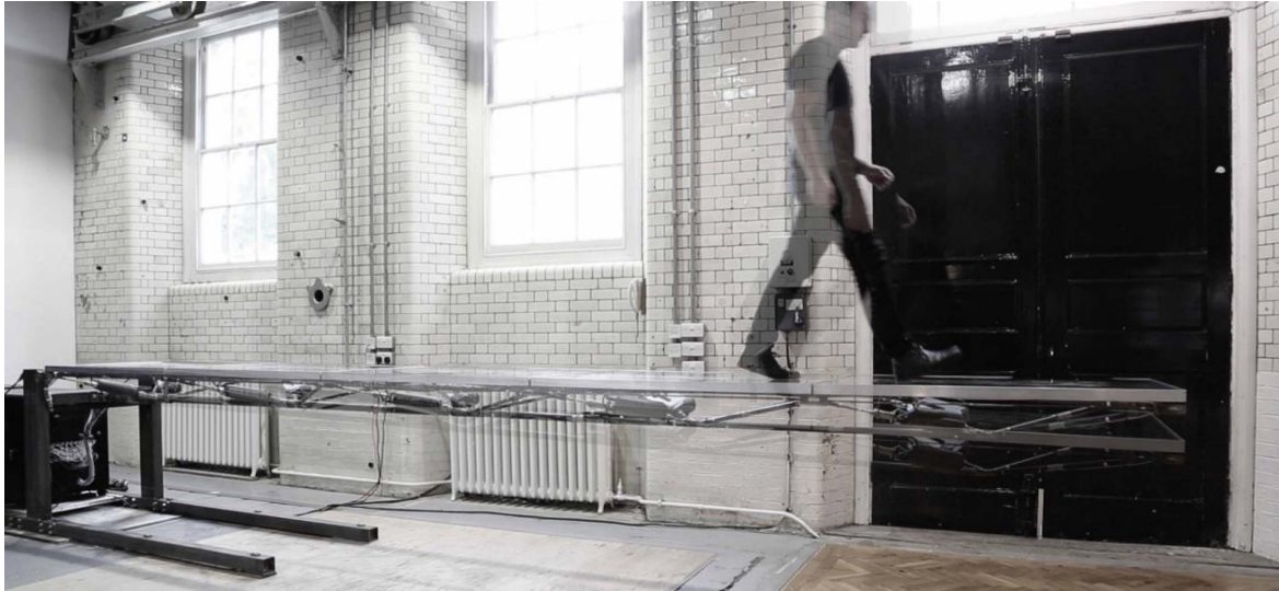
Figure 24. Person (70 kg) walking, comparison deformed (transparent) and controlled shape.
