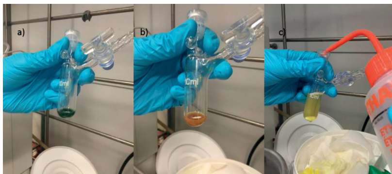
Figure 3.1.7 Change in color of the catalyst upon exposure to air. a) t = 0 s, b) t = 30 s, c) when diluted in EtOH.
