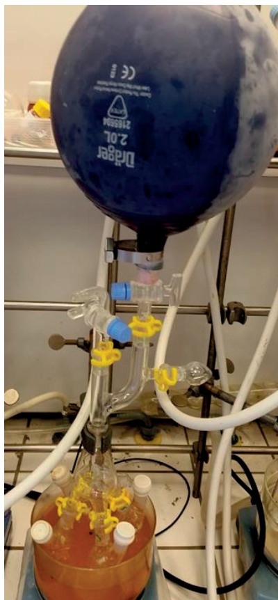
Figure 3.1.5 Photograph of the four parallel reaction apparatus with the distillation distributor and distillation head. No cross-contamination was observed under these conditions.
