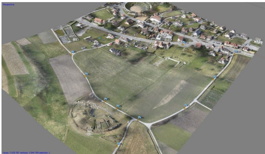
Figure 3: Orthoimage draped on the DTM of Avenches ( Archeotech, EPFL )
