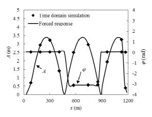
**Figure 12a.** Forced response in the piping system induced by excitation source set to the third hydraulic eigenmode frequency H3 (Hydroelectric system with PSS).
