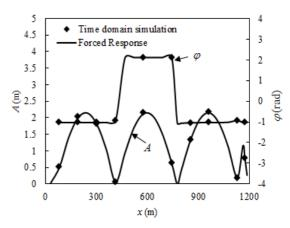
**Figure 12b.** Forced response in the piping system induced by excitation source set to the third hydraulic eigenmode frequency H3 (Hydroelectric system without PSS).
