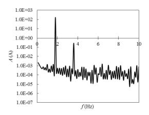
**Figure 7b.** Amplitude spectrum of stator current on phase a in the rotating frame (k) obtained by time domain simulation.
