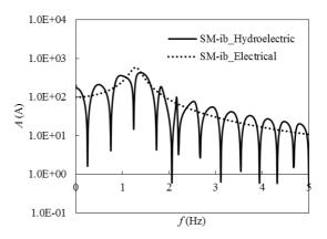
**Figure 11b.** Comparison of the forced response of the synchronous machine obtained with electrical and hydroelectric systems without PSS.
