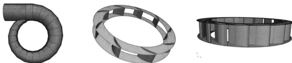
Fig. 2: Structured grids of the spiral casing, the stay vane, the guide vane, the runner and the draft tube
