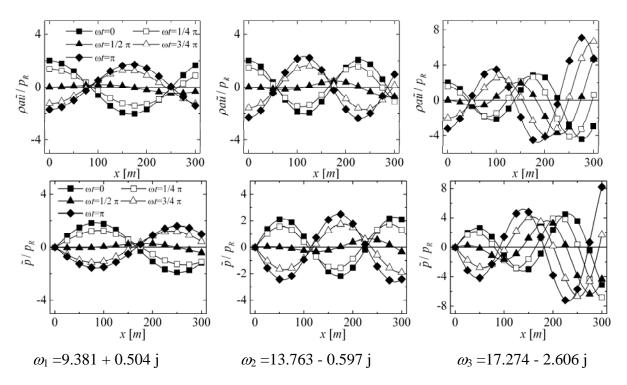
Fig. 6 Velocity and pressure fluctuations along the inlet pipe at  $L_i = 300$  m
