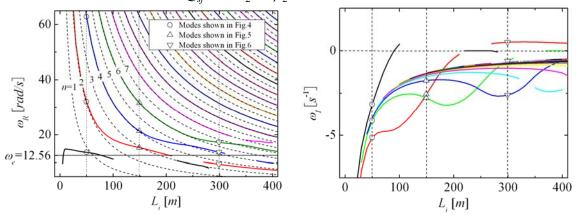
Fig. 3 Higher order frequencies under a = 500 m/s
