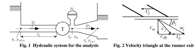
where  $L_e = \int (A_e / A(s)) ds$  is the effective length of the draft tube,  $D = (A_e / A_c)^2 - 1$  the diffuser factor,  $\zeta_2$  the loss coefficient of the draft tube. For simplicity,  $\zeta_2$  is assumed to be constant although it may depend on the swirl of the discharge flow [8]. Equation (2) ignores the flow compressibility in the draft tube.
