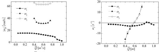
Fig. 8 Effect of  $\overline{Q}$  to first 3 order frequencies at Li = 50 m, under a = 500 m/s
