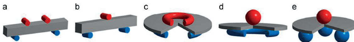
Figure 3: Representation of the most common configurations for bending test of planar samples: a) four-point bending, b) three-point bending, c) ring-on-ring (ROR), d) ball-on-ring (BOR) and e) ball-on-three balls. Figure reproduced from Wei et al. [99] d .
