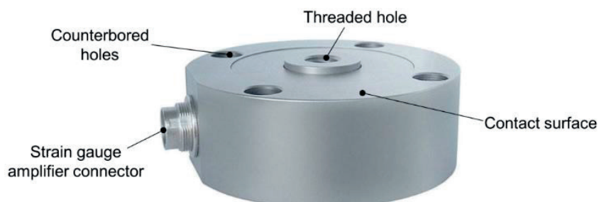
Figure 9: Representation of the load cell model (K11-500N005, Transmetra GmbH) used in the SEP setup. e
