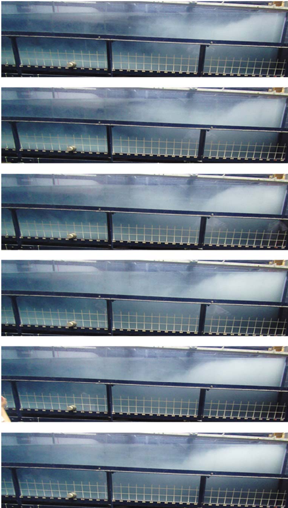
Figure A1.3: Typical behaviour of the turbidity currents for the experimental tests using a slope of 2.4%. Time step \Delta t = 25 s.
