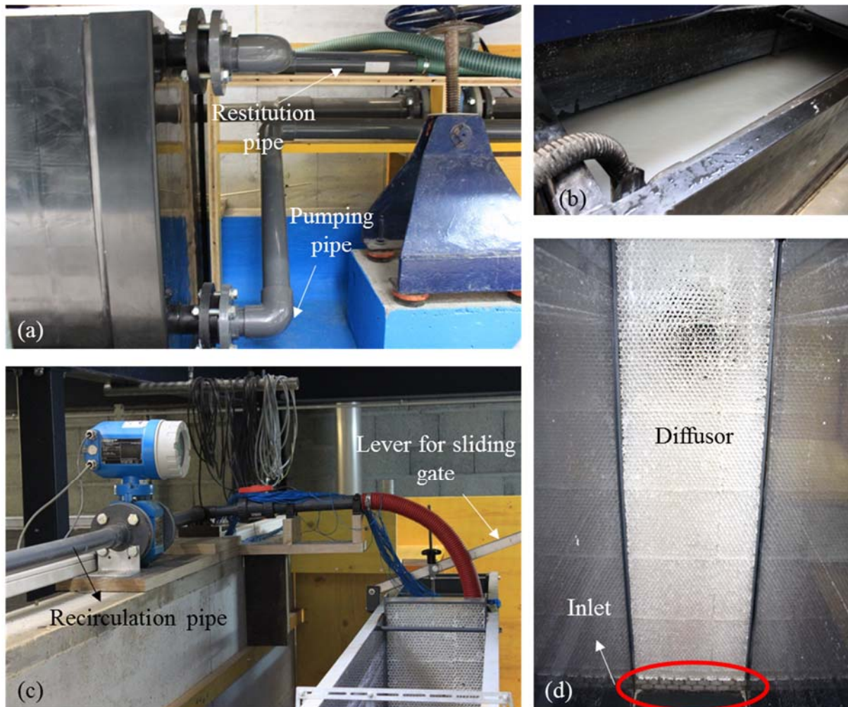
Figure 3.2: (a) The upstream system linking the mixing tank to the head tank, highlighting the restitution and pumping pipes; (b) the mixing tank with the water-sediment mixture inside being mixed by the recirculating pump; (c) system linking the downstream compartment of the flume to the main flume through the recirculation pipe along with the corresponding pump, also showing the lever used to open/close the sliding gate; (d) the inlet and the diffuser above it.
