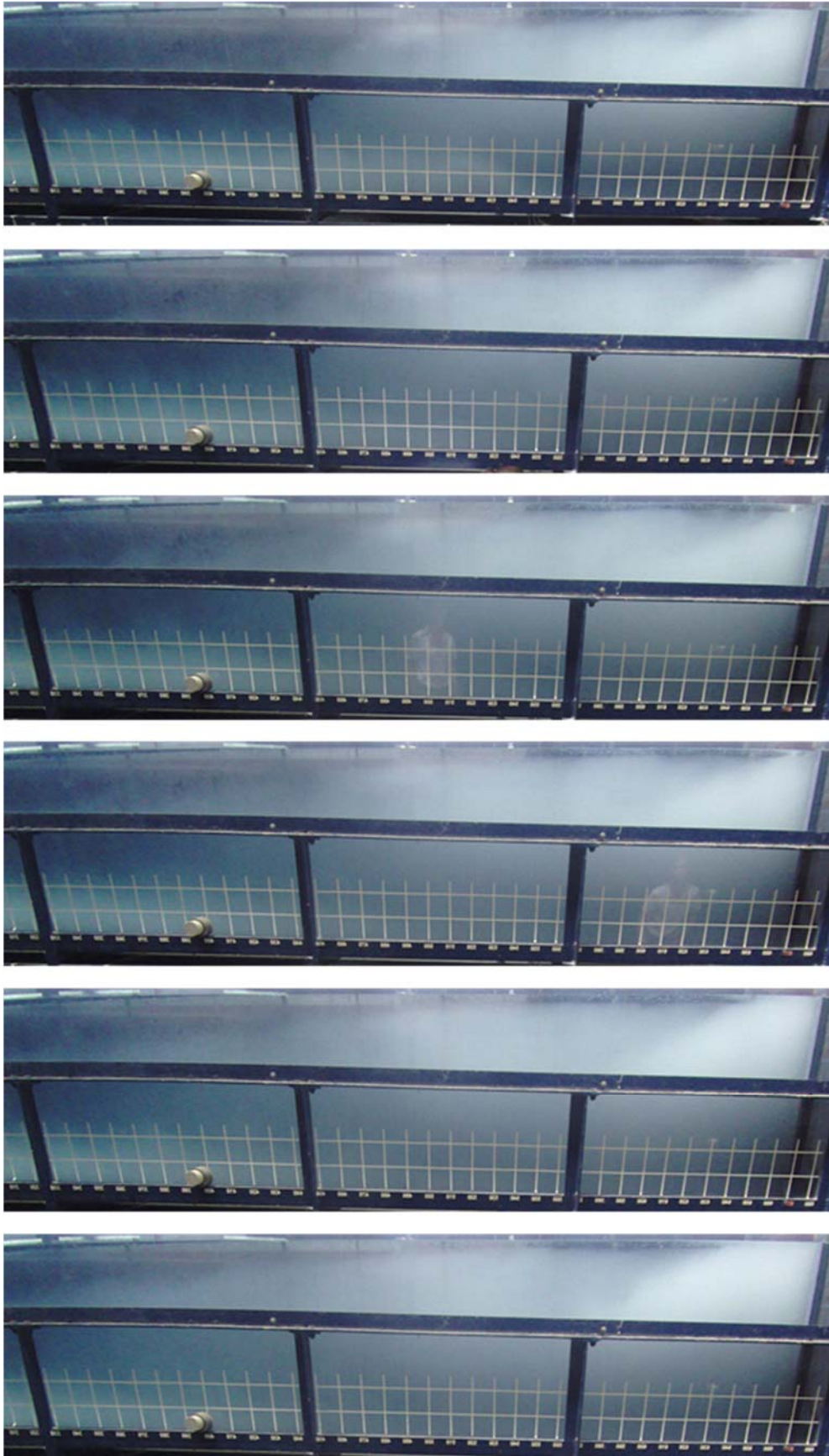
Figure A1.2: Typical behaviour of the turbidity currents for the experimental tests using a slope of 2.4%. Time step \Delta t = 25 s.
