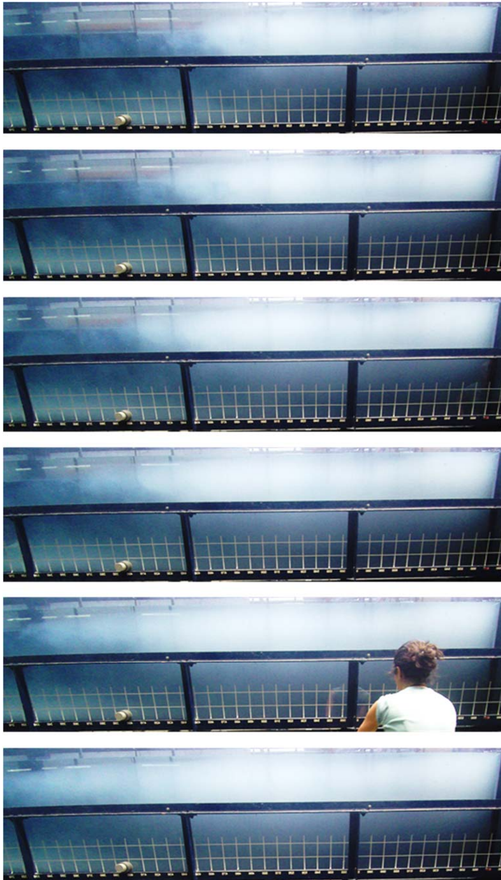
Figure A1.1: Typical behaviour of the turbidity currents for the experimental tests using a horizontal bed. Time step \Delta t = 25 s.
