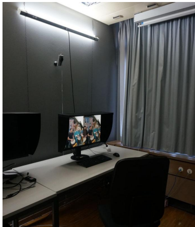
Figure 2. The EPFL test lab setup used during JPEG XS subjective evaluations
