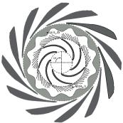
Figure 1: Rotor-Stator interaction between impeller and diffuser
