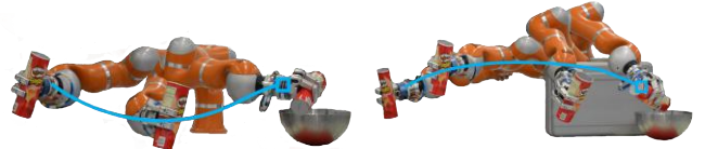
Fig. 1: Two robot motions in joint-space accomplishing similar behavior in task-space (pouring chips in a bowl). The left example avoids a known obstacle in its workspace, while the right one does not.
