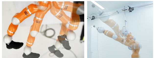
Fig. 7: Execution of problematic joint-space behaviors learned through JT-DS: (left) Foot step-like motion and (right) Singularity motions.
