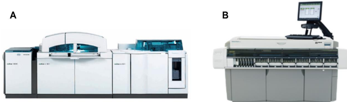
Figure 1.11: Examples of clinical analyzers used nowadays in clinical settings: A) Cobas Integra from Roche Diagnostics B) AxSYM from Abbott Laboratories.
