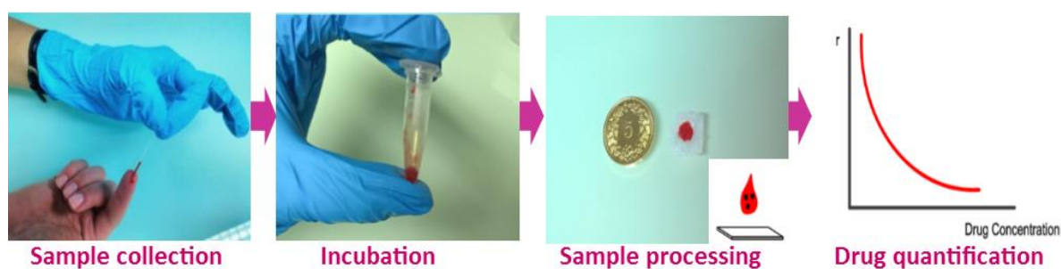
Figure 2.12: Tobramycin quantification within glass fiber micro-chambers at the point-of-care: 1 \mu L of whole blood, which might be obtained from a finger prick and collected using a glass capillary, was mixed with the tracer Atto655-Tob and antibodies against tobramycin. The solution was incubated for 3 minutes before addition of 10 \mu L to the glass fiber micro-chamber and anisotropy read-out at its bottom part.
