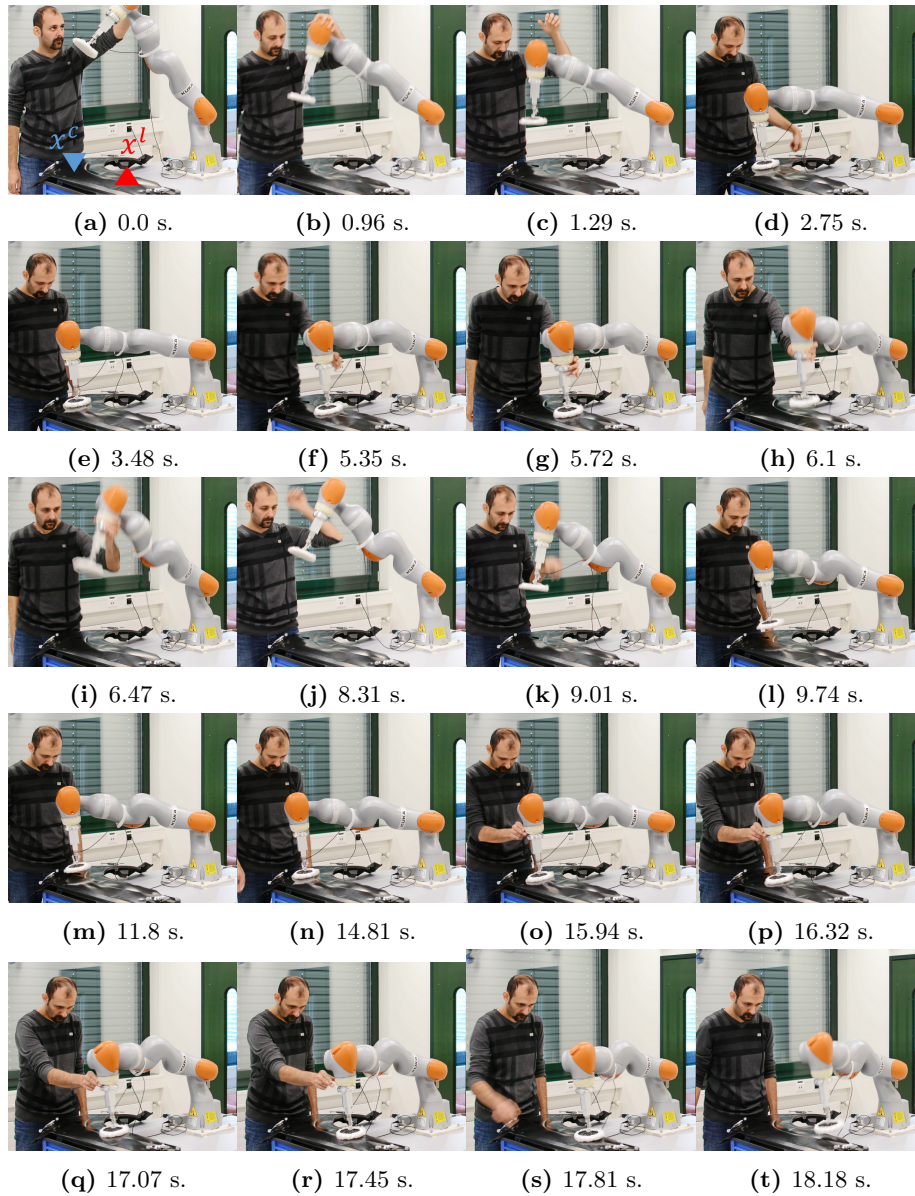
Figure 5.9: Snapshots of the motion of the robot while performing Scenario 1 under perturbations. In (a), the initial configuration of the robot, x^c and x^l are shown.
