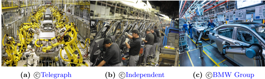
Figure 1.1: Examples of different types of production lines. 1.1a and 1.1b illustrate examples of fully-automated versus fully-manual tasks in a car manufacturer, respectively. In 1.1c, an example of hybrid production line, where a seamless collaboration between humans and robots is essential, is shown.
