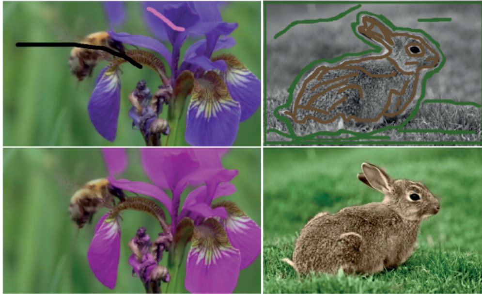
Figure 2.21: Sample results from the interactive image enhancement method [16]. Users draw strokes in different color to indicate the foreground and background, and to assign the colors to the corresponding parts.
