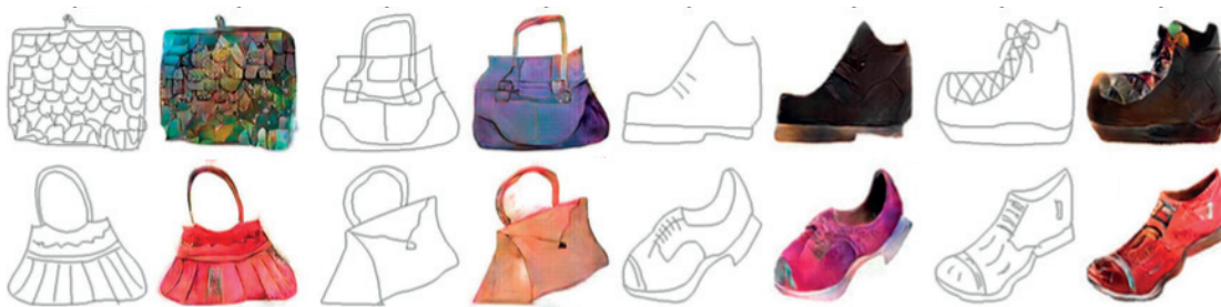
Figure 2.8: Sample results of pix2pix [55] for edge \rightarrow photo application. The network transforms edge images to photos. In each pair, the left one is the edge image and the right one is the generated photos.
