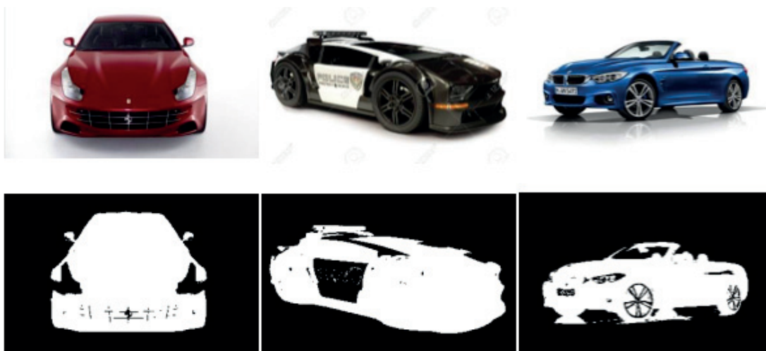
Figure 4.2: Sample images from the white-background set \mathbf{W}_{\text{car}} and the corresponding segmentation masks generated from saliency combined with dense CRFs.
