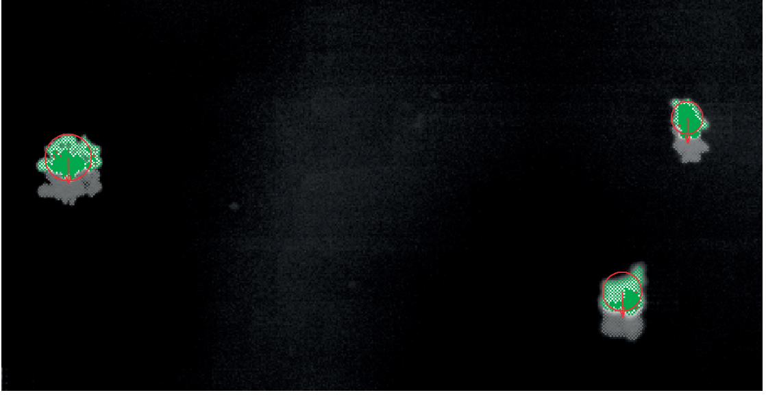
Figure 2.3: The velocity calculation was performed based on the shift between two consecutive images. The green area represents the particle's initial position, the grey area is the final position.
