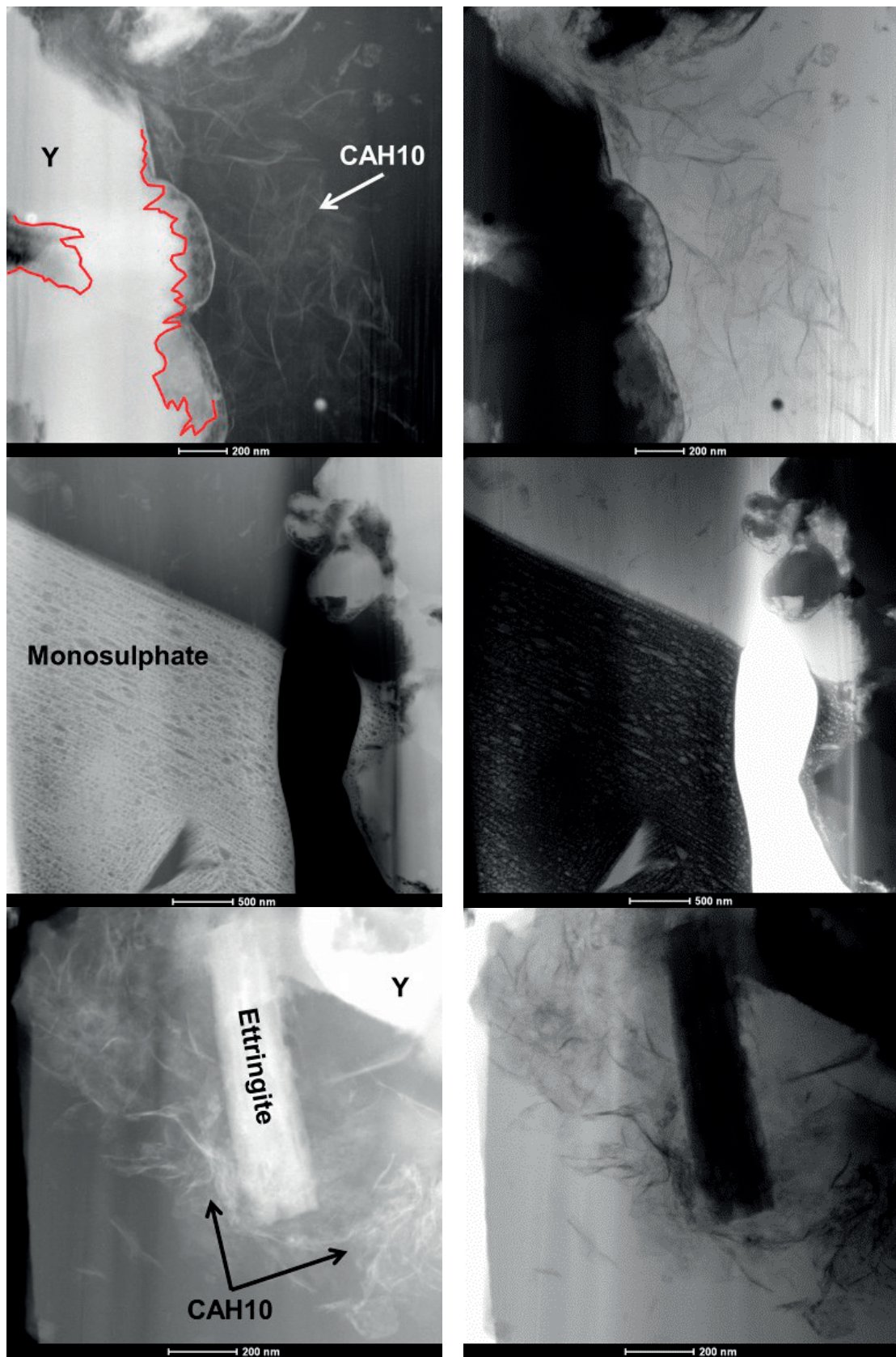
Figure 5.4-8 STEM images (up: HAADF image and down: BF image) of Y after 6 hours of hydration at 23 °C and a w/b ratio of 100; dotted red line indicates the surface of the anhydrous; Y = anhydrous ye'elinite particles
