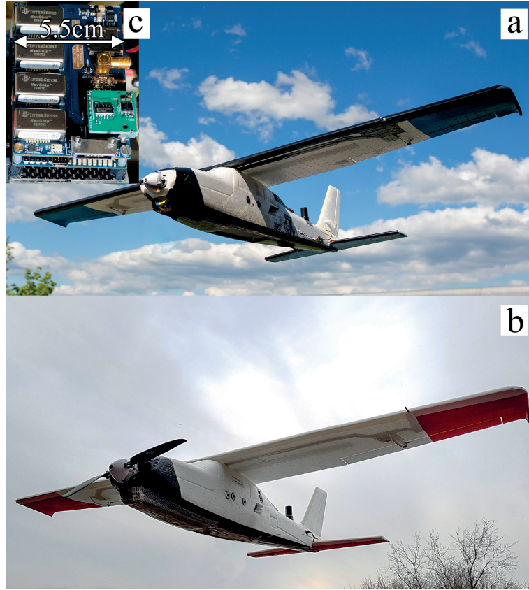
Figure 4.2 – Custom made UAVs, TOPO plane 1 (a) and TOPO plane 2 (b), together with the IMU board (c)
