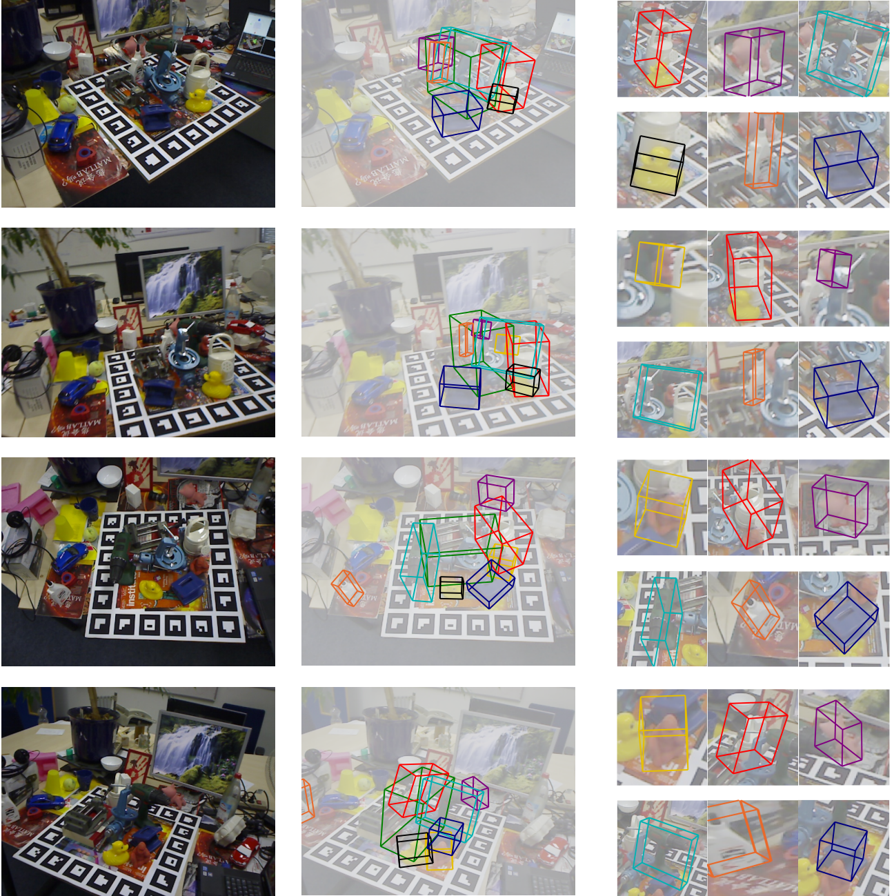
Figure 4. Results on the OCCLUSION dataset. Our method is quite robust against severe occlusions in the presence of scene clutter and rotational pose ambiguity for symmetric objects. (left) Input images, (middle) 6D pose predictions of multiple objects, (right) A magnified view of the individual 6D pose estimates of six different objects is shown for clarity. In each case, the 3D bounding box is rendered on the input image. The following color coding is used – APE (gold), BENCHVISE (green), CAN (red), CAT (purple), DRILLER (cyan), DUCK (black), GLUE (orange), HOLEPUNCHER (blue). In addition to the objects from the OCCLUSION dataset, we also visualize the pose predictions of the Benchvise object from the LINEMOD dataset. As in [7], we do not evaluate on the Eggbox object, as more than 70% of close poses are not seen in the training sequence. This image is best viewed on a computer screen.
