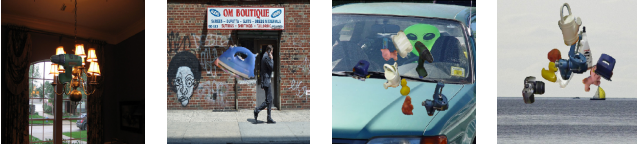
Figure 1. Using segmentation masks given in LINEMOD, we extract the foreground objects in our training images and composite them over random images from PASCAL VOC [4]. We also augment the training set by combining images of multiple objects taken from different training images.
