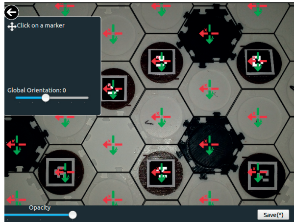
Figure 6.4 – The utility to create the configuration file containing the positions of the fiducial markers.
