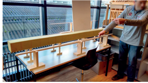
(b) A deformable beam made of glued layers of polyurethane foam.
