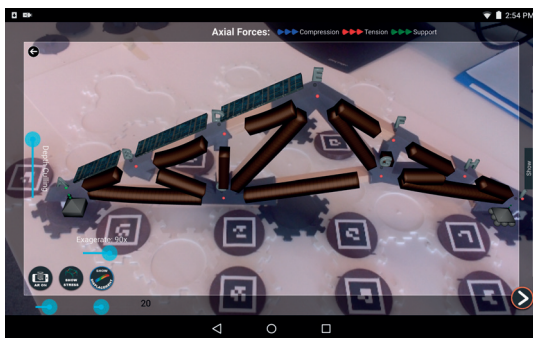
(b) Global deformation of a structure.
