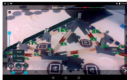
(c) Stresses in the elements of the structure.
