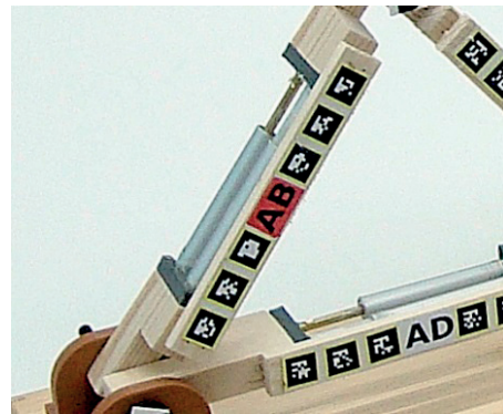
Figure 5.4 – Wooden strip to lock the spring mechanism.
