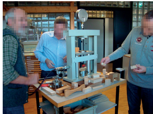
(d) A small hydraulic press to test the strength of several materials.
