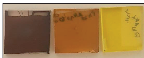
Figure 5.3 Photograph of three different compositions showing the effect of MA/FA ratio (from left to right): \text{FA}_{0.5}\text{MA}_{0.5}\text{PbI}_{2.47}\text{Cl}_{0.53} ; (\text{FAPbI}_3)_{0.85}(\text{MAPbCl}_3)_{0.15} ; (\text{FAPbI}_3)_{0.85}(\text{FAPbCl}_3)_{0.15} .
