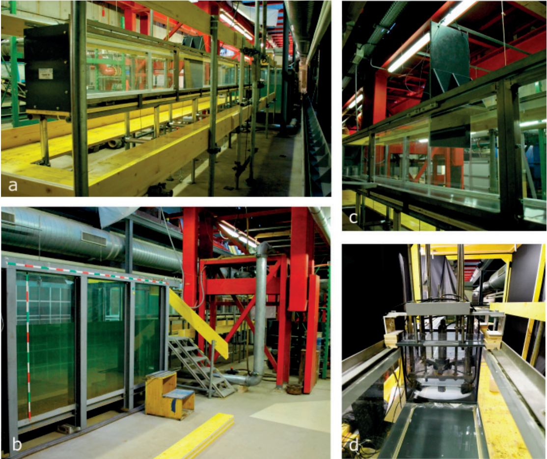
Figure 3.2: Experimental set-up at the Laboratoire de Constructions Hydrauliques (LCH) of EPFL with the upstream tank (a), the downstream reservoir (b), the gate (c) and the Acoustic Doppler Velocity Profiler (d) instrument for velocity measurements.
