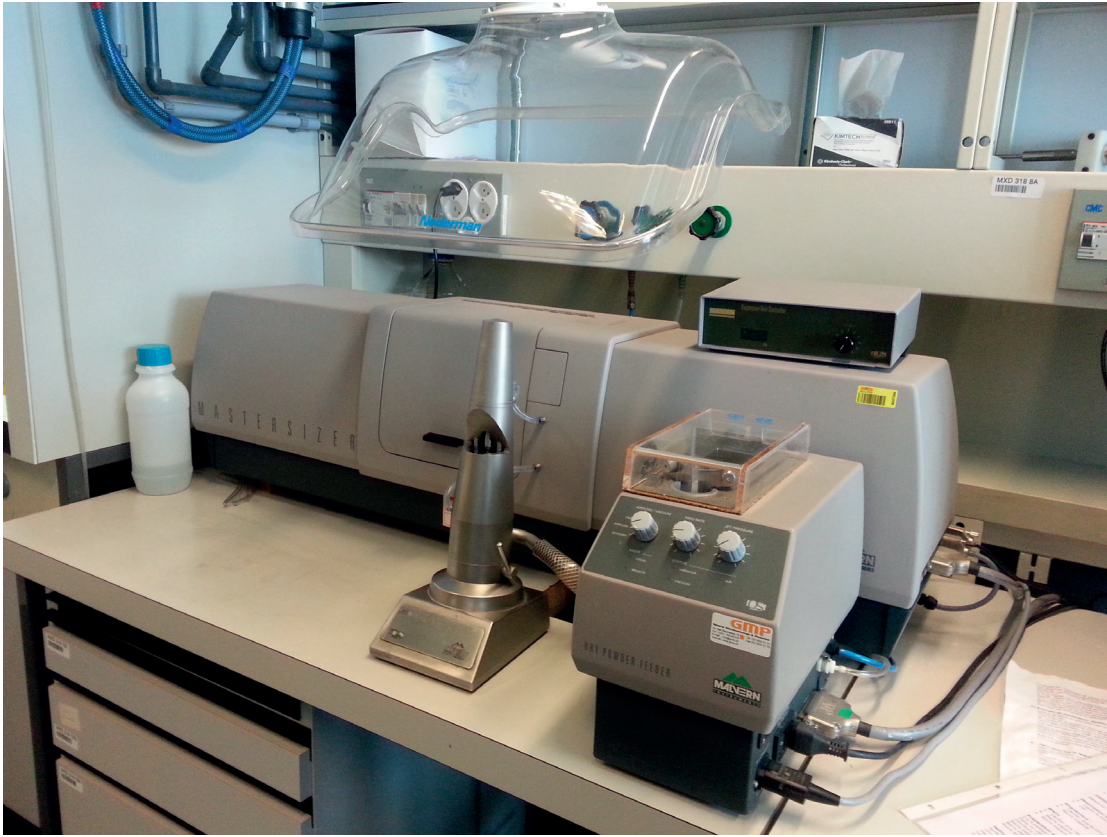
Figure C.1: The Malvern Master sizer laser diffraction particle size analyser at Laboratoire de technologie des poudres (LTP) of the EPF Lausanne.
