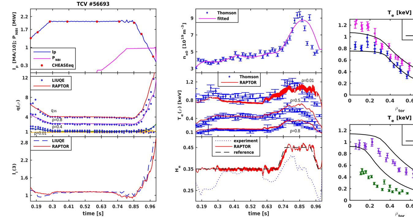
**Prescribed parameters:** the total plasma current I, radial profiles of the electron density n, the total input NBI power with central deposition and the prescribed Gaussian radial profile, H<sub>2</sub>=0.35/0.45 and  $\lambda_{2}$ =3.2/2.3 for L-/H-mode.
