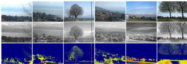
Figure 2. Dehazing masks (bottom) obtained by comparing the NIR information (middle) with the visible images (top) for images from the dataset provided by [6].
