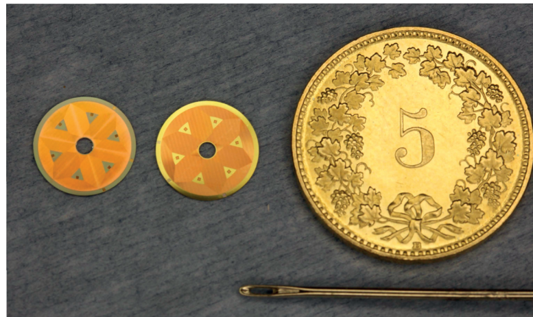
Figure 5.22 – Completed stators with adhesion layers in SiO 2 (left) and Al (right).
