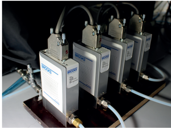
Figure 2:7 Mass flow controllers used to control the atmosphere in the sample holders. Each of these can be connected to a different gas and a precise flow rate can be programmed.
