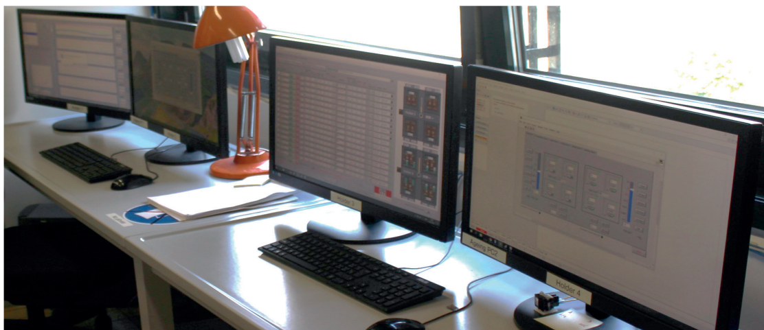
Figure 2:13 Picture of the “command and control center” of the stability measurement setup. Each PC is connected to two monitors and is used to control half of the setup (2 holders, 1 potentiostat, 1 control box).
