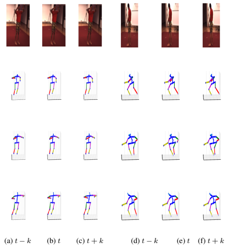
Fig. 10 Pose estimation results with LSTMs on Human3.6m. (a,d) t - k^{th} frame. (b,e) t^{th} frame. (c,g) t + k^{th} frame. k denotes the stride between consecutive frames. Top row: Input image, Second row: Our pose estimate from the single image, Third row: Our BLSTM pose estimate, Last row: Ground truth. Our BLSTM network can correct for the errors made by the autoencoder by accounting for the temporal consistency. Best viewed in color.
