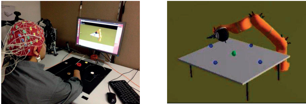
Figure 2.9: Decoding goal from slow cortical EEG signals on left which moves the KUKA robot arm optimally to the desired target on right.
