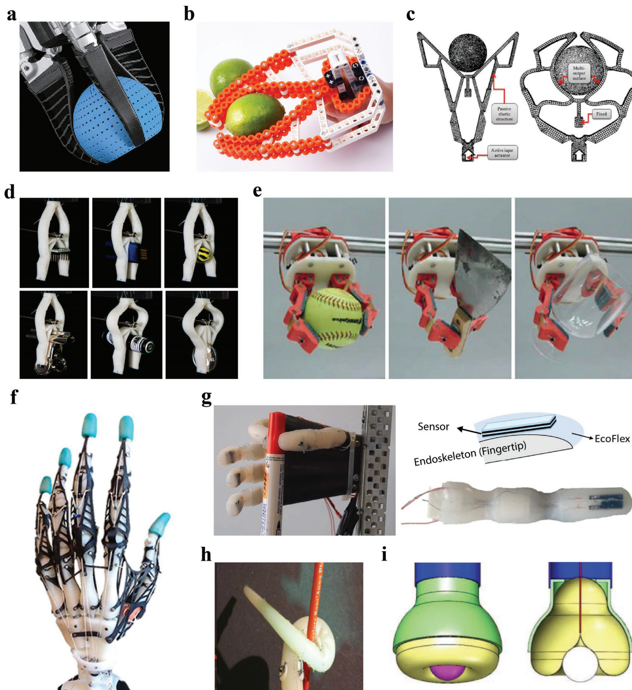
Figure 4. Soft grippers using passive structure with external motors. a) Fin Ray robotic gripper. [11] Reproduced with permission. Copyright Festo AG & Co. KG. b) Fin Ray (toy). Reproduced with permission. [16] Copyright BionicToys GmbH. c) Working principle of compliant mechanism. Reproduced with permission. [28] Copyright 2013, Emerald Publishing. d) Compliant mechanism. Reproduced with permission. [30] Copyright 2017, Springer Nature. e) Tendon-driven with elastic hinges. Reproduced with permission. [50] Copyright 2017, IEEE. f) Anthropomorphic tendon-driven. Reproduced with permission. [54] Copyright 2016, IEEE. g) Tendon-driven with sensor embedded soft skin. Reproduced with permission. [59] Copyright 2017, IEEE. h) Tendon-driven elastomeric manipulator. Reproduced with permission. [67] Copyright 2011, IOP Publishing. i) Tendon-driven with a compliant elastomeric bag. Reproduced with permission. [63] Copyright 2016, IEEE.
