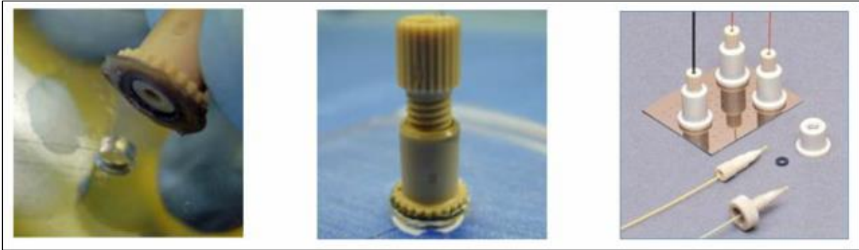
Fig. 51: Examples of NanoPorts. The ring can be seen on the left; mounted NanoPort attached to the chip on the center; NanoPorts with tubing shown on the right [39].
