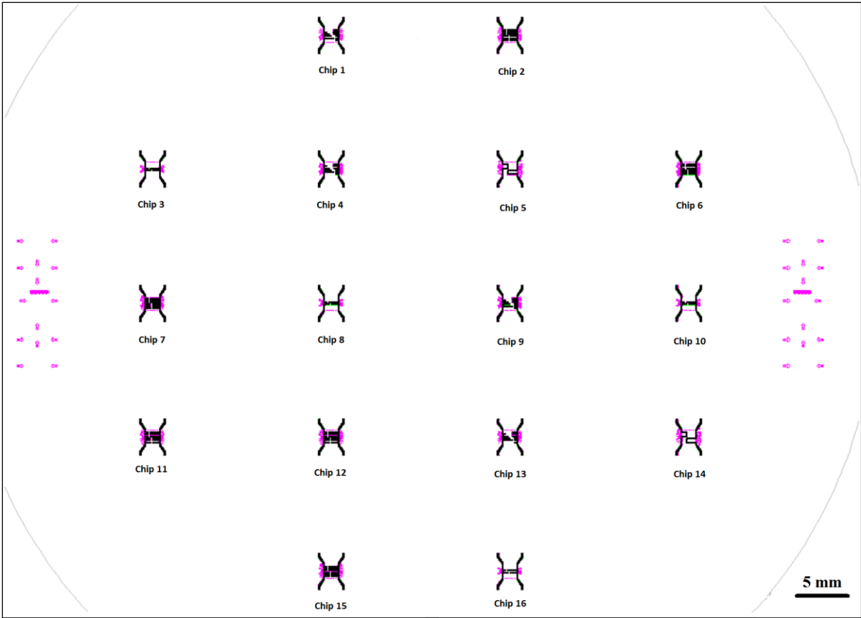
Fig. 19: Wafer layout showing the 16 chips. Image from CleWin.
