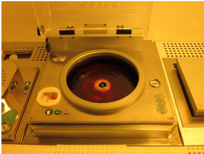
Fig. 33: ATMsse OPTIspin used for coating. The hotplate used for softbake is on the right [34].
