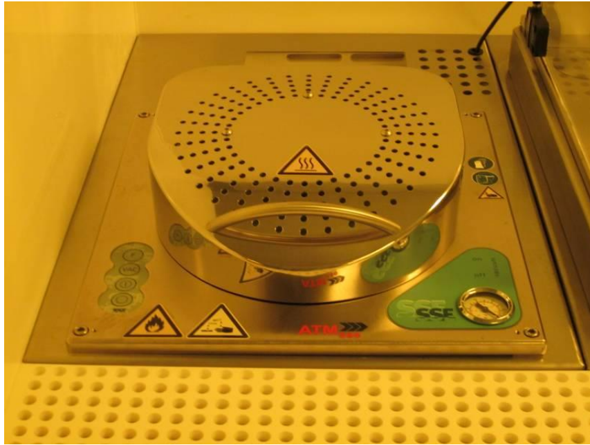
Fig. 32: ATMsse OPTIhot tool used for surface preparation [33].
