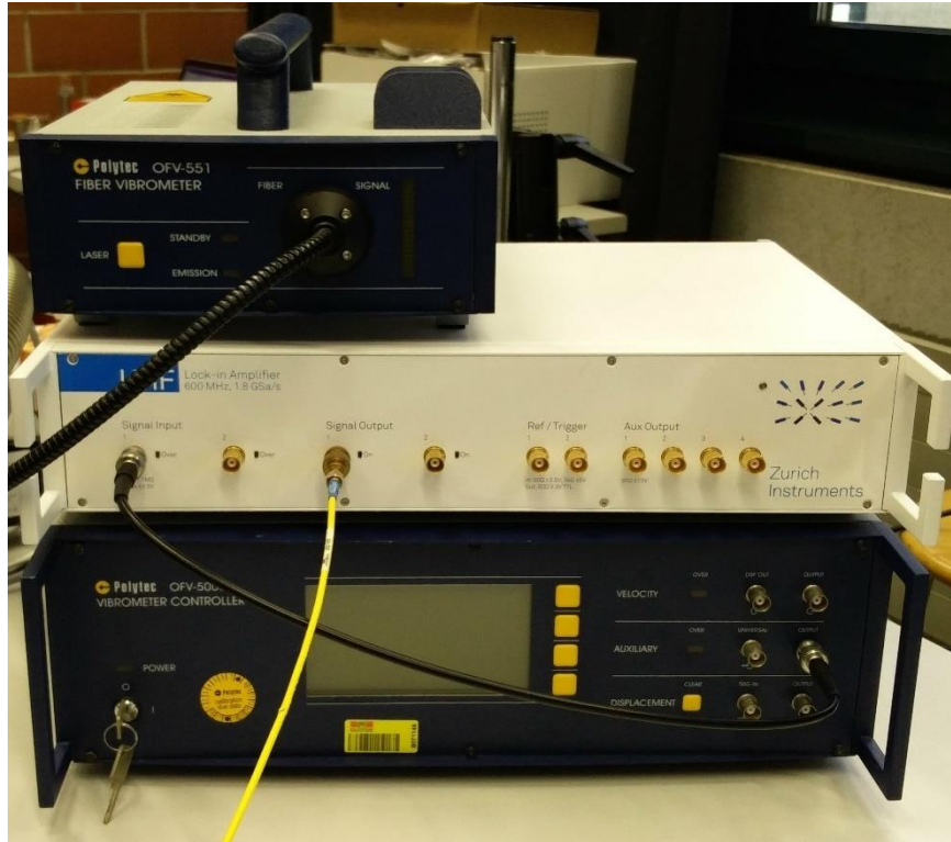
Fig. 57: Sensor head, vibrometer controller and lock-in amplifier. The yellow cable from the amplifier is connected to the piezo crystal, while the fiber optic from the sensor head goes to the microscope.
