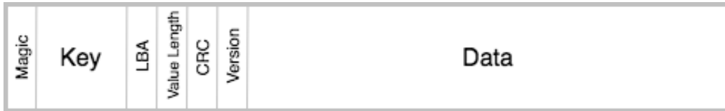
Figure 4.1: The metadata components of a block.
