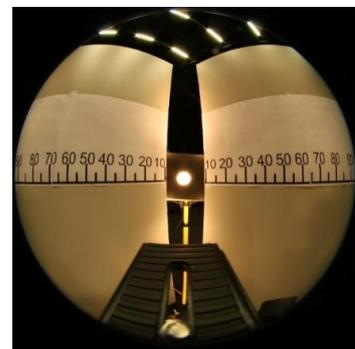
Figure 3: The vignetting setup with the camera pointing at the source.
