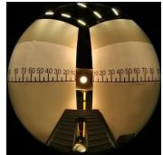
Figure 3: The vignetting setup with the camera pointing at the source.
