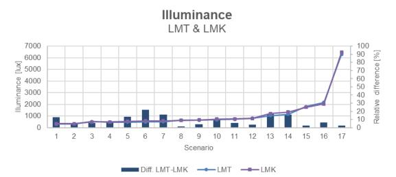
Figure 8: Illuminance values measured with the LMT meter and calculated from the LMK camera. The bars show percentage difference and follow the right-hand axis.
