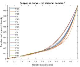
Figure 1: The red channel response curves for camera 1 for all the apertures.
