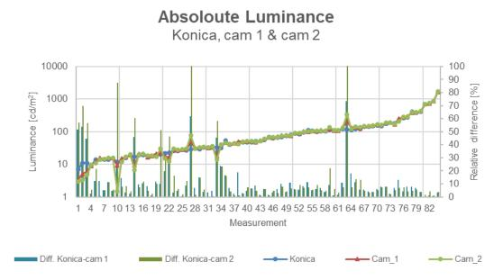
Figure 9: Luminance values measured with the Konica Minolta and DSLR cameras. The bars show percentage difference and follow the right-hand axis.
