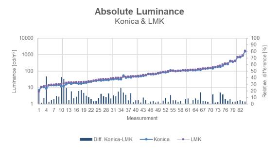
Figure 7: Luminance values measured with the Konica Minolta and LMK luminance camera. The bars show percentage difference and follow the right-hand axis.
