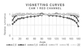
Figure 4: A selection of vignetting curves from different apertures for the red channel of camera 1.
