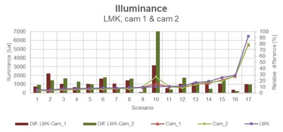
Figure 12: Illuminance values calculated from the LMK and DSLR cameras. The bars show percentage difference and follow the right-hand axis.
