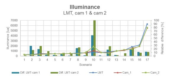
Figure 10: Illuminance values measured with the LMT meter and calculated from the DSLR cameras. The bars show percentage difference and follow the right-hand axis.
