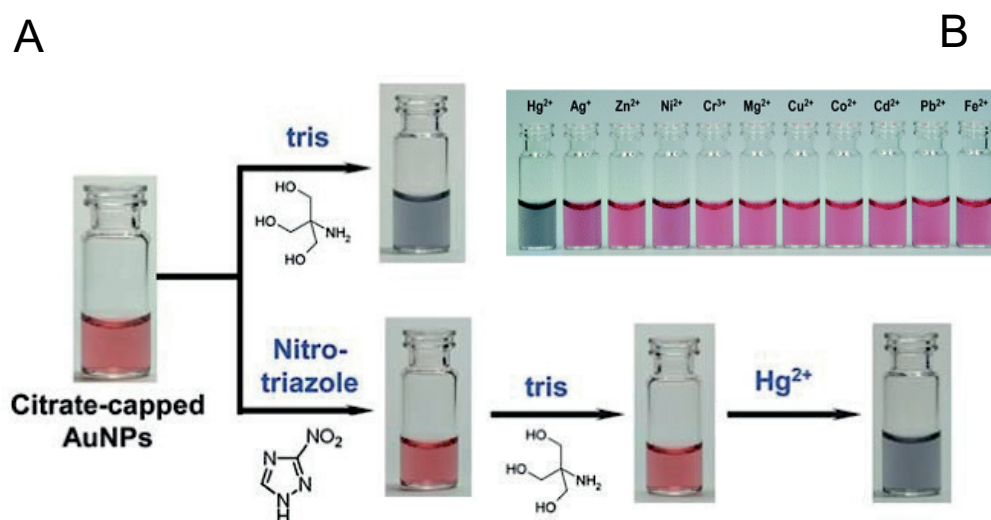
Figure 1.6: A) Color changes of the citrate-capped AuNPs upon the addition of Tris buffer, NTA, and Hg 2+ , respectively. B) Color changes of the NTA-AuNP probes upon the addition of various metal ions. Adapted from Ref. 46 with permission from The Royal Society of Chemistry.
