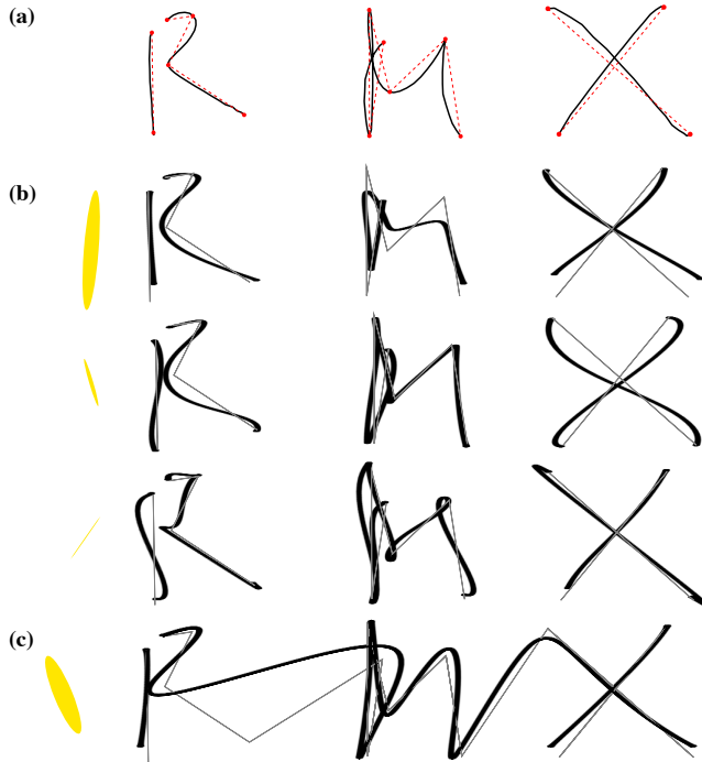
Figure 10: Handwritten letter stylisation. (a) Traces taken from the UIJI data set and the corresponding target positions (automatically generated). (b) Different stylisations are achieved by using different semi-tied covariance settings. (c) Generation of smooth ligatures. NB: for illustrative purpose we chose a rather low angle threshold of 100^\circ .
