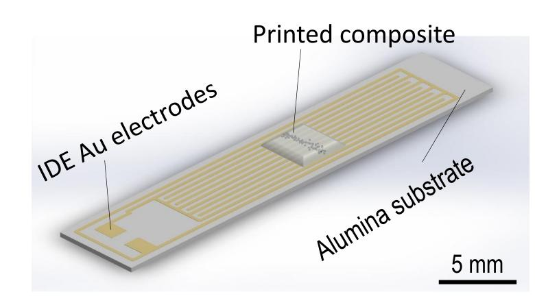
Schematic of the sensor platform with screen printed IDE
