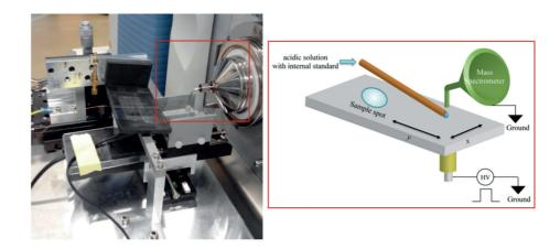
**Figure 1.15.** Schematic representation of the setup for ESTASI-MSI. Figure from Anal. Chem., **2014**, 86, 2033-2041.
