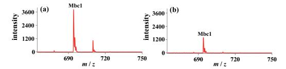
**Figure 4.4. (a)** and **(b)** MALDI mass spectra of 1 nM Mbc1-coded AuNPs with and without DHB as matrix, respectively. The spectra were acquired under positive mode with an accelerating voltage of 19 kV, a 20 Hz repetition rate, the laser intensity of  $\sim 40\%$  (instrumental value) and an average of 800 shots.
