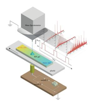
**Figure 1.10.** Schematic representation of ESTASI-MS coupled with IEF-GE. Figure from Anal. Chem., **2013**, 85, 4745-4752.
