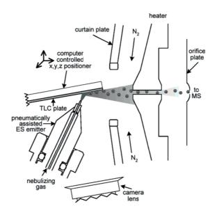
**Figure 1.9.** Schematic illustration of the TLC/DESI-MS. Figure from Anal. Chem., 2005, 77, 1207-1215.
