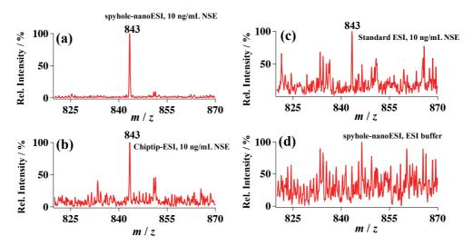
**Figure 5.8.** NSE detection by single reaction monitoring (SRM) of its signature peptide SP-14. 10 ng/mL NSE tryptic digest in ESI buffer (50% MeOH, 49% H<sub>2</sub>O and 1% acetic acid) was used for the following tests. Mass spectra of the signature fragment ion of SP-14 at m/z 843.4 obtained by (a) spyhole-nanoESI MS/MS; (b) chiptip-ESI MS/MS; (c) standard ESI MS/MS. (d) Mass spectrum of the ESI buffer obtained by spyhole-nanoESI MS/MS.
