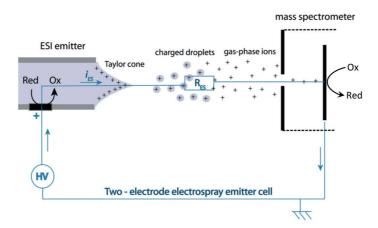
**Figure 1.5.** Classical electrospray ionization process. Figure from Annu. Rev. Anal. Chem., **2010**, 3, 231-254.
