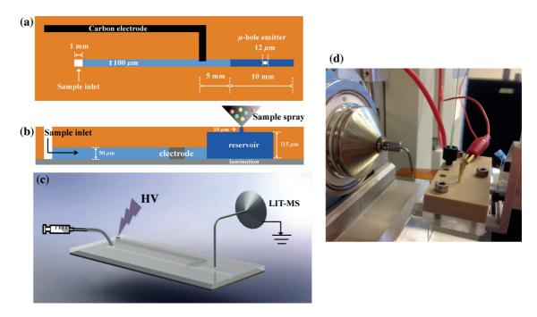
**Figure 5.1.** Schematic representation of the spyhole-nanoESI device: (a) top-view image, (b) side-view image, (c) 3D image, and (d) real picture on a plastic holder. The holder was fixed onto an x, y, z positioning stage and placed horizontally under an "L-shaped" MS ion transfer capillary. HV: high voltage. LIT-MS: linear ion trap mass spectrometry.
