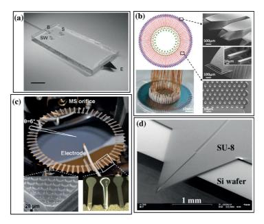
**Figure 1.13.** ESI for coupling microfluidic chips with MS from integrated emitters of: (a) a graphite-coated PDMS microchip tip, (b) a 96-capillary array, (c) a platform with 60 silicon microchip tips, and (d) nib-like tips fabricated using the negative photoresist SU-8. Figure (a) from Electrophoresis, **2005**, 26, 4674-4683; figure (b) from Anal. Chem., **2011**, 83, 6082-6089; figure (c) from Lab Chip, **2011**, 11, 3011-3014; figure (d) from Electrophoresis, **2003**, 24, 3640-3647.
