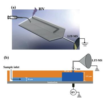
**Figure 5.2.** Schematic representation of different devices: (a) 3D image of chiptip-ESI and (b) sideview image of spyhole-nanoESTASI. HV: high voltage. LIT-MS: linear ion trap mass spectrometry.
