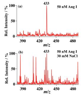
**Figure 3.6.** The test of ESTASI tolerance to salt by the analysis of  $10 \,\mu\text{L}$  50 nM Ang I in the well of a 384-well plate. The buffer of 50% methanol, 49% H<sub>2</sub>O and 1% acetic acid contains (a) no salt or (b) 30 mM NaCl.
