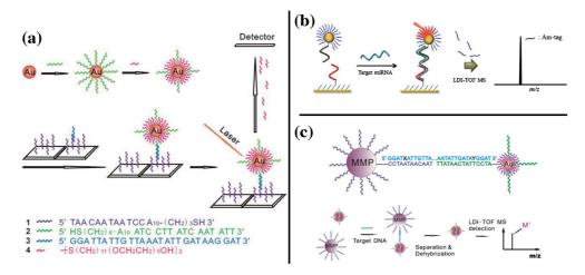
**Figure 1.2.** Mass barcoded AuNPs and AuMPs for DNA sensing on different surfaces: **(a)** silica wafer chip, **(b)** gold chip, and **(c)** magnetic beads. Figure (a) from Angew. Chem. Int. Ed., **2008**, 47, 5009-5012; figure (b) from Analytical Biochemistry, **2013**, 434, 199-201; figure (c) from Talanta, **2011**, 85, 1698-1702.
