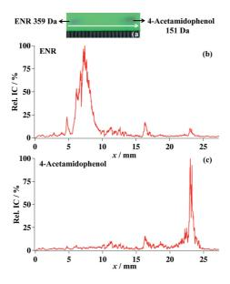
**Figure 2.11.** ESTASI-MS line-scan of a drug mixture containing ENR (1.4 nmole) and 4-acetamidophenol (3.3 nmole) on a silica gel TLC plate with silane modification. (a) an optical image of the dried sample spots on the TLC plate. (b) and (c) Rel. IC/% chromatography of ENR and 4-acetamidophenol, respectively.
