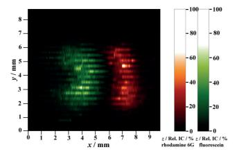
**Figure 2.6.** 2D TLC-ESTASI-MSI of rhodamine 6G and fluorescein spots in Figure 2.5(a). Rel. IC/% of each dye was plotted with respect to the position on the TLC plate and represented individually as the z-axis in a form of green (fluorescein) or red (rhodamine 6G) colour gradient.
