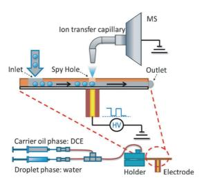
**Figure 1.14.** On-chip spyhole coupled with ESTASI-MS for droplet-based microfluidics. Figure from Angew. Chem., **2014**, 126, 4497-4501.
