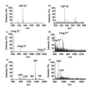
**Figure 3.2.** Mass spectra obtained by the 384-well plate ESTASI-MS of (a) 1.5  $\mu$ M of CIP, (b) 15 nM of CIP, (c) 15  $\mu$ M of Ang I, (d) 15 nM of Ang I, (e) 10  $\mu$ M of Cyt c and (f) 100 nM of Cyt c. Solution: 50% MeOH/49% H<sub>2</sub>O/1% acetic acid. CIP+H<sup>+</sup>: singly protonated CIP; (Ang I)<sup>x+</sup>: Ang I ion with x proton(s); XH<sup>+</sup>: Cyt c ion with x proton(s).
