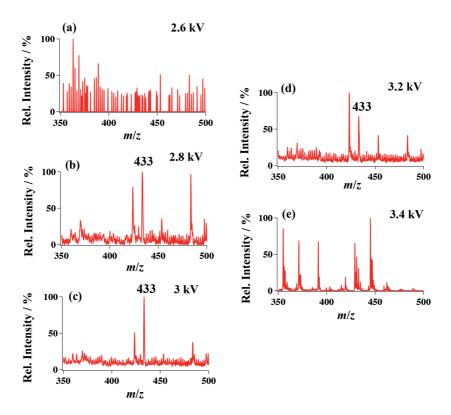
**Figure 5.4.** Analyses of 0.15 nM Ang I in ESI buffer by spyhole-nanoESI MS with voltages of: (a) 2.6 kV, (b) 2.8 kV, (c) 3 kV, (d) 3.2 kV and (e) 3.4 kV. AGC target value was set as 10'000. The other detection conditions were the same as those given in experimental part of 5.2.2.
