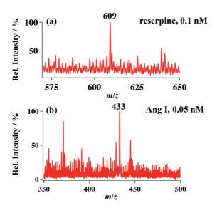
**Figure 5.6.** Detection of different molecules in ESI buffer (50% MeOH, 49%  $H_2O$  and 1% acetic acid) by the spyhole-nanoESI MS: (a) 0.1 nM reserpine, (b) 0.05 nM Ang I. The detection conditions were the same as the optimized one given in experimental part of 5.2.2.
