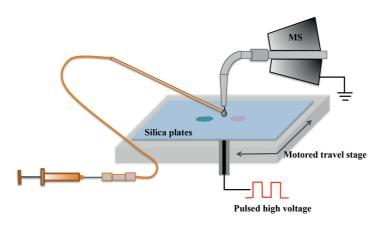
**Figure 2.1.** Schematic representation of the setup used for TLC-ESTASI-MS.
