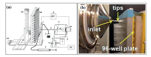
**Figure 1.11.** MS coupled with microtiter plates. (a) Direct-infusion with a capillary from microtiter plates for ESI-MS analysis; (b) Microtiter plates modified with multiple pipette tips for high throughput solvent assisted inlet ionization (SAII) MS analysis. Figure (a) from Anal. Chem., **2001**, 73, 1449-1454; figure (b) from Anal. Chem., **2014**, 86, 1000-1006.
