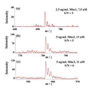
**Figure 4.9.** MALDI mass spectra of the mass barcodes: 1  $\mu$ L of (a) 2.5 ng/mL Mbc1, (b) 5 ng/mL Mbc2, and (c) 5 ng/mL Mbc3. 0.5  $\mu$ L of 10 mg/mL DHB was used as the matrix.
