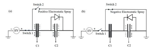
**Figure 1.8.** Equivalent circuit of the ESTASI during the charging-discharging process. Figure from Anal. Chem., **2012**, 84, 7422-7430.
