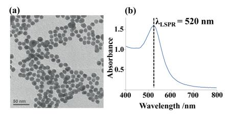
Figure 4.1. (a) TEM image of synthesized AuNPs. (b) UV-Vis spectrum of the synthesized AuNPs.
