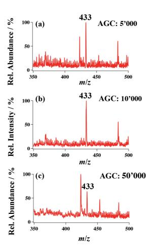
**Figure 5.5.** Analyses of 0.15 nM Ang I in ESI buffer by spyhole-nanoESI MS with AGC values of: **(a)** 5'000, **(b)** 10'000 and **(c)** 50'000. Voltage: 3 kV. The other detection conditions were the same as those given in experimental part of 5.2.2.
