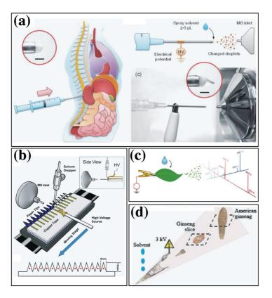
**Figure 1.7.** Different sampling probes for ESI: (a) Needle biopsy on tissue for direct ESI; (b) High-throughput paper spray-MS Platform; (c) Leaf for direct ESI; (d) Wetted ginseng tissue for ESI. Figure (a) from Anal. Chem., **2011**, 83, 9221-9225; figure (b) from Clin. Chim. Acta., **2013**, 420, 28-33; figure (c) from Anal. Chem., **2011**, 83, 7608-7613; figure (d) Rapid Commun. Mass Spectrom., **2011**, 25, 2837-2843.
