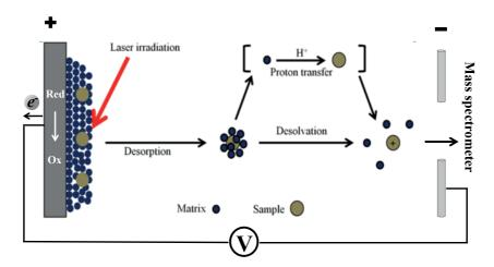
**Figure 1.1.** Schematic representation of a MALDI source in positive ionization mode. Figure adapted from "Mass Spectrometry: Principles and Applications", 3<sup>rd</sup> edition, de Hoffmann *et al.*, John Wiley & Sons Ltd. © 2007.
