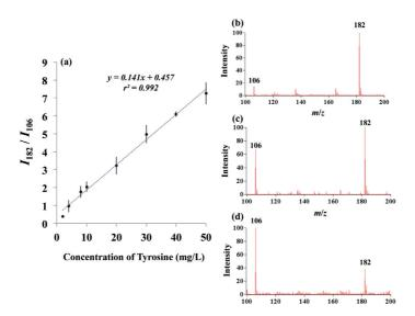
**Figure 3.3.** (a) Liner curve fitted for tyrosine quantification with internal standard calibration method.  $I_{182}/I_{106}$ : relative ion intensities between tyrosine ( $I_{182}$ ) and serine ( $I_{106}$ ). (b), (c) and (d) Mass spectra for 50 mg/L, 8 mg/L and 2 mg/L of tyrosine, respectively. The analyses were performed with direct ESTASI-MS from a 384-well plate, each well containing 10  $\mu$ L of analyte solution in 50%
