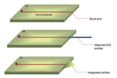
**Figure 1.12.** ESI for coupling microfluidic chips with MS from: **(a)** a blunt-end chip, **(b)** an attached emitter, and **(c)** an integrated emitter. Figure from J. Mass. Spectrom., **2009**, 44, 579-593.
