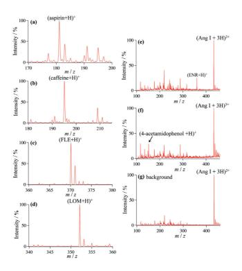
**Figure 2.12.** (a), (b), (c) and (d) individual ESTASI-MS spectra of aspirin (2.7 nmole), caffeine (2.6 nmole), FLE (1.3 nmole) and LOM (1.4 nmole), respectively. (e), (f) and (g) mass spectra obtained at x = 7 mm, x = 23 mm and x = 14 mm, respectively, of Figure 2.11. (Drug + H)<sup>+</sup>: singly protonated drug; (Ang I + 3H)<sup>3+</sup>: triply protonated Ang I.
