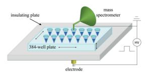
**Figure 3.1.** Schematic representation of the setup used for ESTASI-MS from a 384-well plate. HV: high voltage, which is a square wave pulsed HV here.
