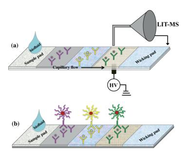
**Figure 6.1**. Direct coupling of ESTASI-MS with lateral flow tests. **(a)** High throughput analyses of multiple target analytes from biofluids captured and separated on a lateral flow strip. **(b)** Amplified ESTASI-MS signals with various mass barcoded particles for multiplex analyses of biofluids.
