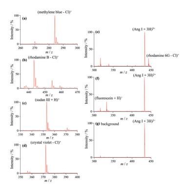
**Figure 2.4.** (a), (b), (c) and (d) individual ESTASI-MS spectra of methylene blue (1.7 nmole), rhodamine B (1.1 nmole), sudan III (1.4 nmole) and crystal violet (1.3 nmole), respectively. (e), (f) and (g) mass spectra obtained at x = 7.5 mm and y = 3 mm, x = 4.5 mm and y = 4 mm, x = 5.5 mm and y = 7 mm, respectively, of Figure 2.6. (Dye + H)<sup>+</sup>: singly protonated dye; (Dye - Cl)<sup>+</sup>: dechlorinated dye; (Ang I + 3H)<sup>3+</sup>: triply protonated Ang I.
