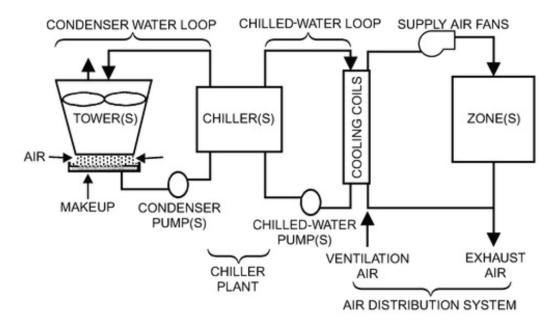
Figure 2.1 – Prototypical cooling system. From [24]
