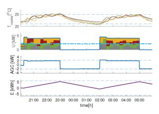
Figure 5.1 – Validation of virtual storage concept. (Upper: Zone temperature (different colors denote the temperatures in different zones), Middle Up: Power distribution among zones (different colors denote the distribution of power in different zones), and nominal consumption (dotted blue), Middle Down: Extra power input to the building with respect to the nominal consumption, Lower: Energy content of the extra power input to the building)
