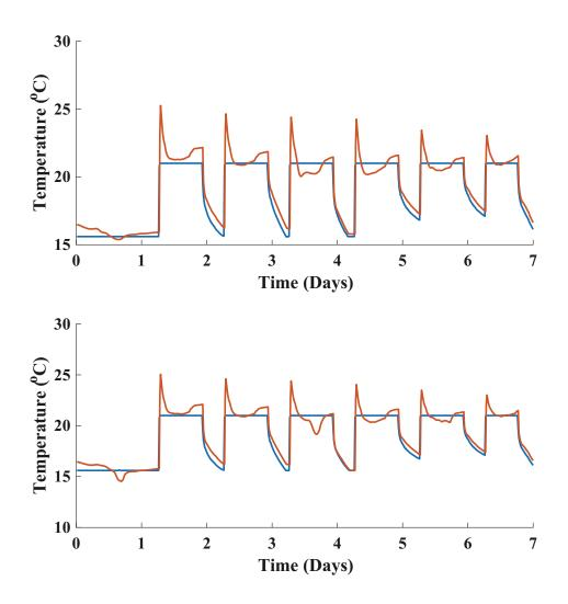
Figure 3.5 – Open loop output comparison - Small Office (zone 1 (top), zone 2 (bottom): EnergyPlus - Blue, OpenBuild model - Red)
