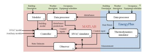
Figure 3.2 – Dataflow in OpenBuild co-simulations
