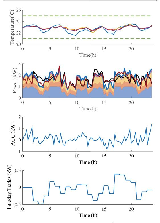
Figure 5.2 – Closed Loop Control for AGC Tracking - day 1 (top: zone temperatures - different colors correspond to temperatures in different zones, middle up: total power **e** (blue), original baseline  $\mathbf{\bar{e}}$  (black), modified baseline  $\mathbf{\bar{e}} + \gamma \mathbf{\bar{m}}$  (red), middle down: AGC  $\gamma \mathbf{a}$ , bottom: intraday trades  $\gamma \mathbf{\bar{m}}$ .
