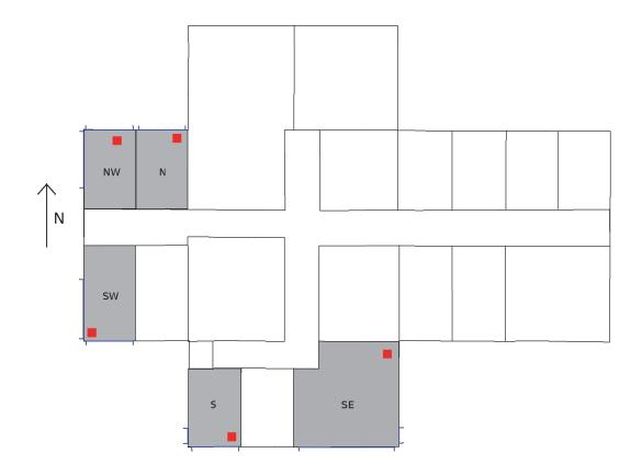
Figure 7.1 – Floor map of the offices used in LADR. The offices shaded in grey have been equipped with sensors and electric radiators and used for experiments. Red squares show the position of the heating units.
