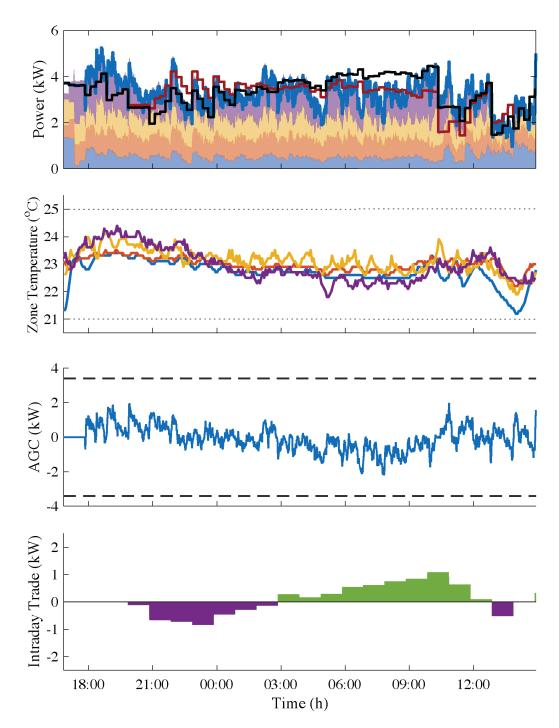
Figure 7.6 – Experiment of AGC tracking with Intraday participation - day 1. top: total power (blue), effective baseline (black), day-ahead baseline (red) and power distribution among zones, middle-up: zone temperatures - different colors correspond to temperatures measured in different zones, middle down: AGC, bottom: intraday trades.
