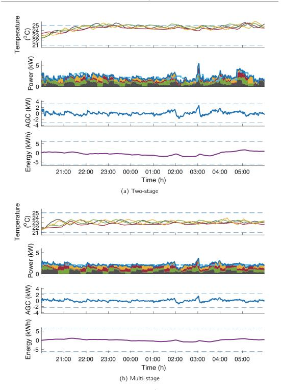
Figure 7.4 – Two experiments of AGC tracking. 1<sup>st</sup> selected AGC signal extracted from real data of 2013, and is used to test and compare the two controllers. Upper: Temperature variation for different zones. Each color corresponds to the measured temperature in each zone. Middle Up: Baseline and power distribution among zones. Middle Down: AGC signal variation and capacity bid. Lower: Integral of the AGC.
