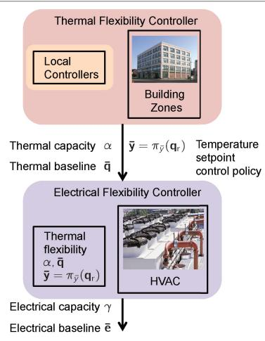
Figure 8.1 – Hierarchical Control Architecture: Bidding/Offline phase. See Table 8.1 for Symbol definition.
