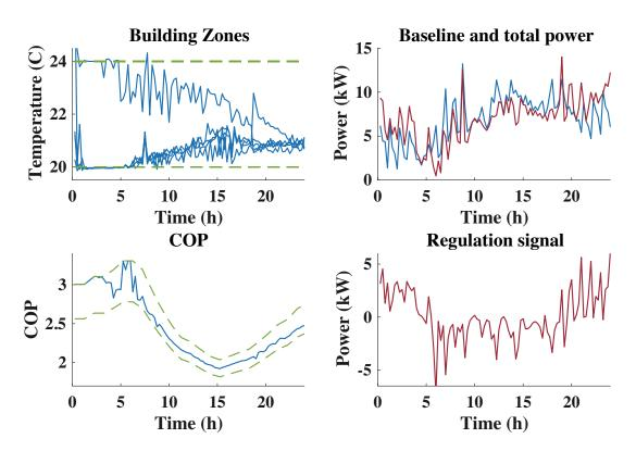
Figure 8.6 – Electrical Flexibility Validation - Varying supply temperatures. Top left: Zone temperatures. Top right: Electrical power  $\mathbf{e}_{ch}$  (red), and baseline  $\mathbf{e}_{b}$  (blue). Bottom left: COP. Bottom right: Regulation Signal **r** (dashed green lines denote operational constraints).
