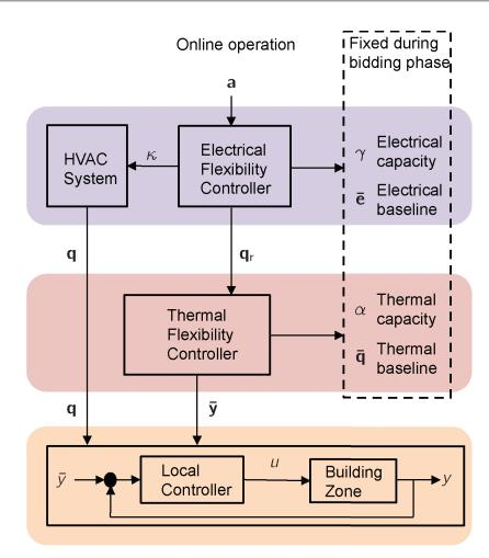
Figure 8.2 - Hierarchical Control Architecture: Online operation phase. See Table 8.1 for Symbol definition.
