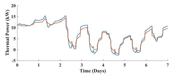
Figure 3.7 – Open loop input comparison - Small Office: EnergyPlus - Blue, OpenBuild model - Red)
