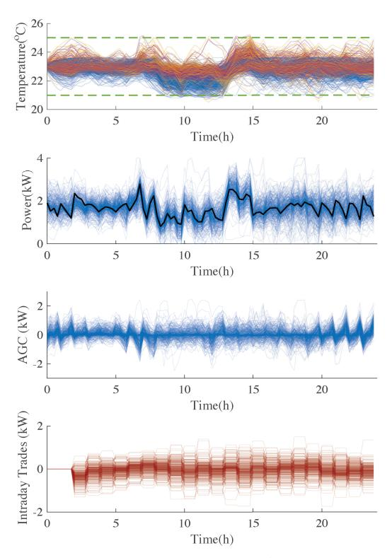
Figure 5.4 – Closed Loop Control for AGC Tracking - yearly (top: zone temperatures on different days of the year - different colors correspond to temperatures in different zones, middle up: original baseline  $\mathbf{\bar{e}}$  (black), total power consumption on different days of the year  $\mathbf{\bar{e}} + \gamma \mathbf{r}$  (blue), middle down: AGC  $\gamma \mathbf{a}$ , bottom: intraday trades  $\gamma \mathbf{m}$ .
