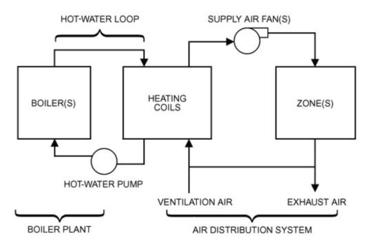
Figure 2.2 – Prototypical heating system. From [24]
