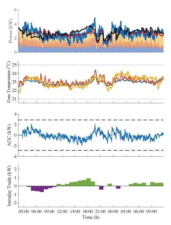
Figure 7.7 – Experiment of AGC tracking with Intraday participation - day 2. top: total power (blue), effective baseline (black), day-ahead baseline (red) and power distribution among zones, middle-up: zone temperatures - different colors correspond to temperatures measured in different zones, middle down: AGC, bottom: intraday trades.
