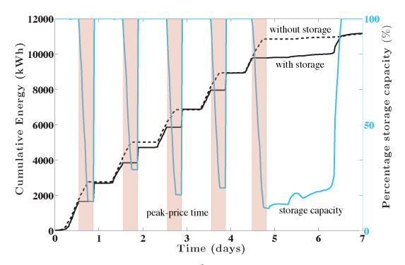
Figure 3.13 – Impact of storage  $(30m^3)$  on building's cumulative energy use
