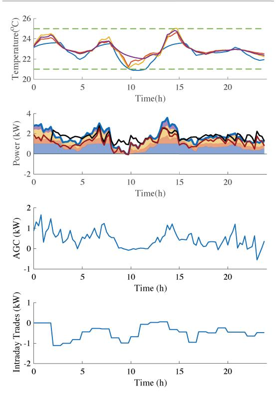
Figure 5.3 – Closed Loop Control for AGC Tracking - day 2 (top: zone temperatures - different colors correspond to temperatures in different zones, middle up: total power **e** (blue), original baseline  $\mathbf{\bar{e}}$  (black), modified baseline  $\mathbf{\bar{e}} + \gamma \mathbf{\bar{m}}$  (red), middle down: AGC  $\gamma \mathbf{a}$ , bottom: intraday trades  $\gamma \mathbf{\bar{m}}$ .
