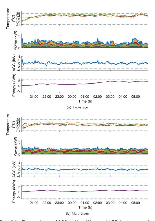
Figure 7.5 – Two experiments of AGC tracking. 2<sup>nd</sup> selected AGC signal extracted from real data of 2013, and is used to test and compare the two controllers. Upper: Temperature variation for different zones. Each color corresponds to the measured temperature in each zone. Middle Up: Baseline and power distribution among zones. Middle Down: AGC signal variation and capacity bid. Lower: Integral of the AGC.
