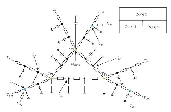
Figure 3.1 - Model Structure (green nodes: zone air, blue node: outside surfaces, black nodes: inside surfaces)
