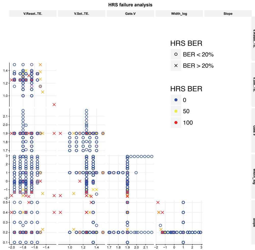
Figure 5.12 – Scatterplot matrix showing the relation between the input test parameters and the HRS BER. The quantities varied during the analysis are the reset voltage, set voltage, gate voltage, pulse width and pulse slope. The x-axis is common for all the plots on the same column, while the y-axis is in common for all the plots in the same row.
