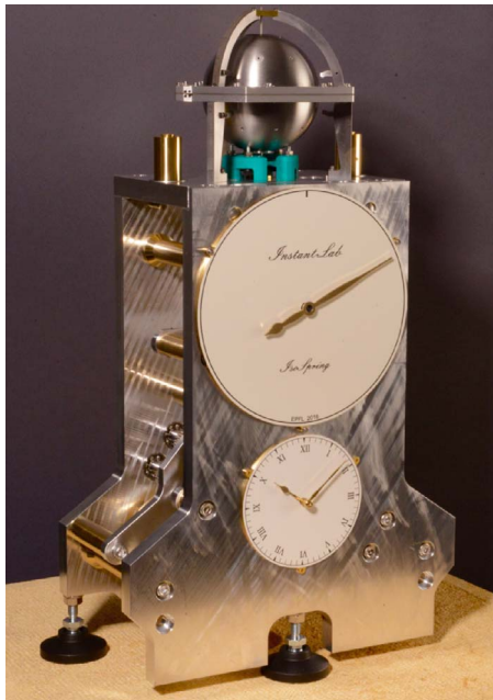
Fig. 1. Clock with time base our spherical oscillator.
