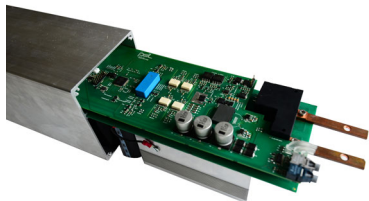
▲ MMC Cell - metal enclosure
