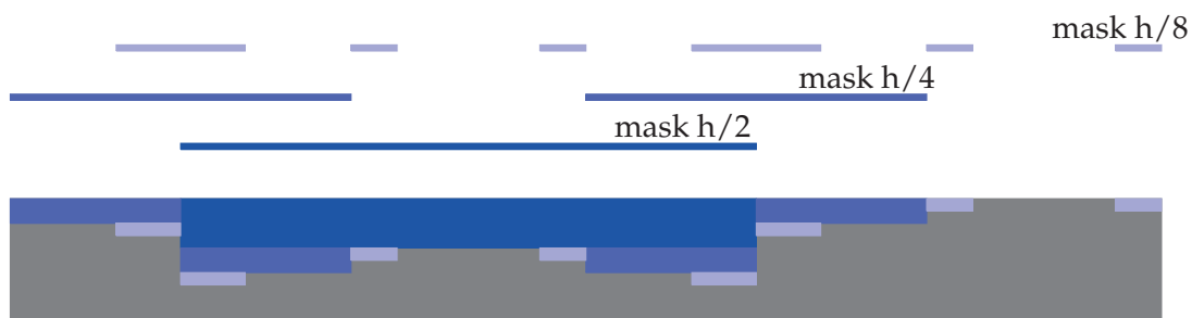
Figure 5.15: Multilevel fabrication of element F with a period of 50\ \mu\text{m} . 3 Masks were used for the fabrication, which is illustrated above the wafer. The structures of each mask are etched with different etch depths. First, the mask with the smallest etch depth h/8 was etched, then the second highest etch depth h/4 and last the highest etch depth h/2 . The height h refers to the depth, for which a phase difference of 2\pi can be achieved.
