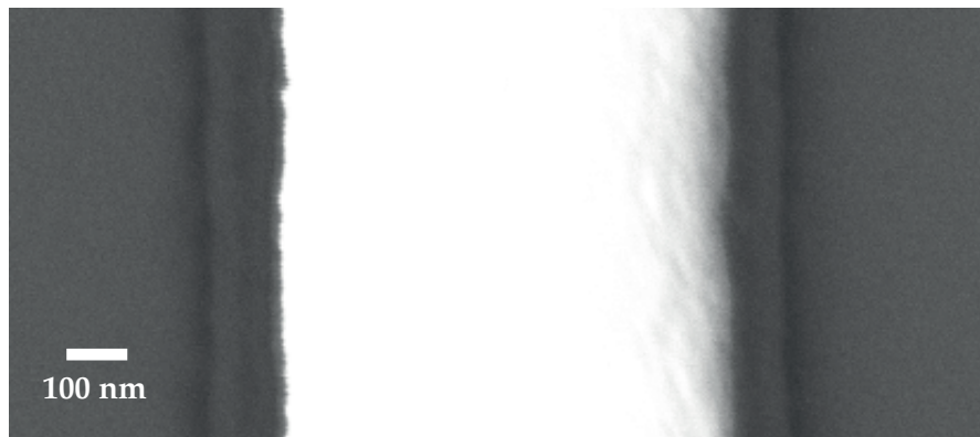
Figure 3.20: SEM image of the photoresist is taken without an Au coating, which decreases the resolution. The photoresist is after development not perfectly straight.
