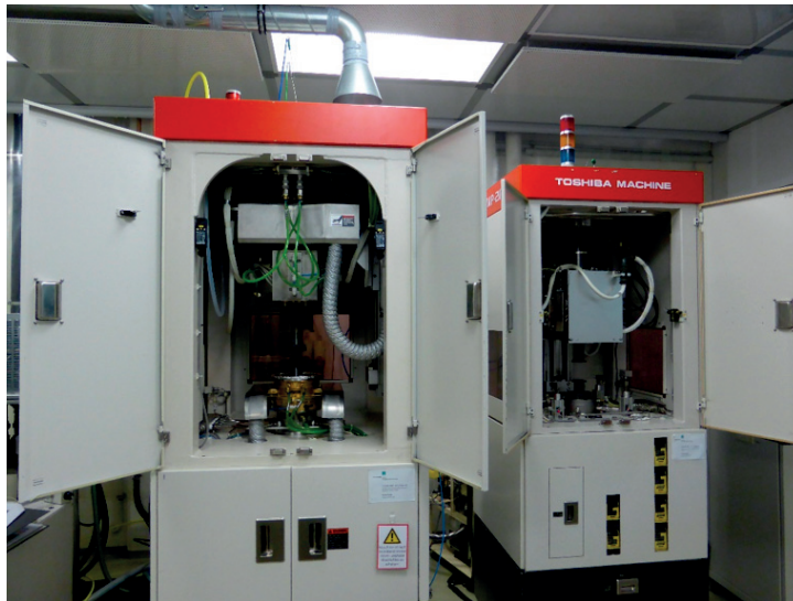
Figure 4.1: Molding machines at IPT Aachen (Germany): (left) Toshiba GMP-207HV ( T \leq 1400 °C) and (right) Toshiba GMP-211V ( T \leq 800 °C)
