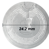
Figure 2.16 – The indoors localization passive tag
