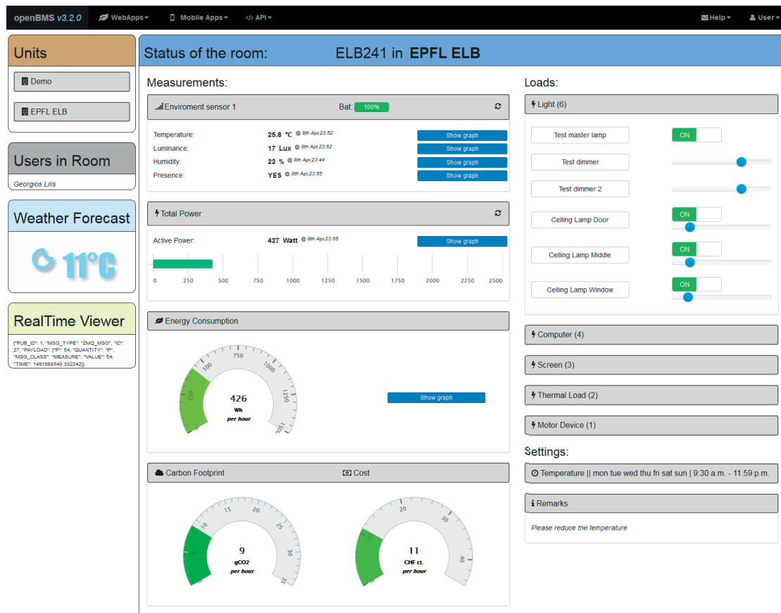
Figure 2.5 – An example frontend as a minimal BMS dashboard
