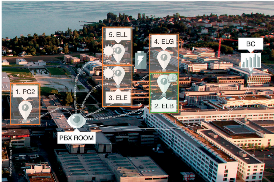
Figure 5.1 – The EPFL "Smart Grid Campus Project", in green the smart building and orange the PMU locations
