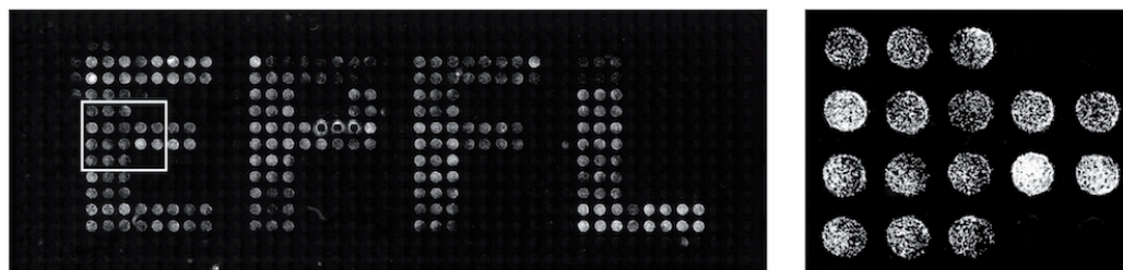
Figure 2.9. Fluorescence micrograph of an entire 675-well acrylic array in which some of the wells were spotted with tdTomato-expressing 3T3 fibroblasts by simultaneously using three spotting pins. Boxed region of the array is magnified on the right.
