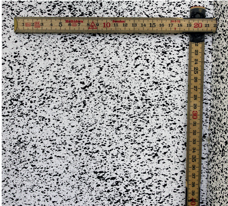
Figure 3.14 – Speckle pattern with speckle sizes between 1 – 5 mm.
