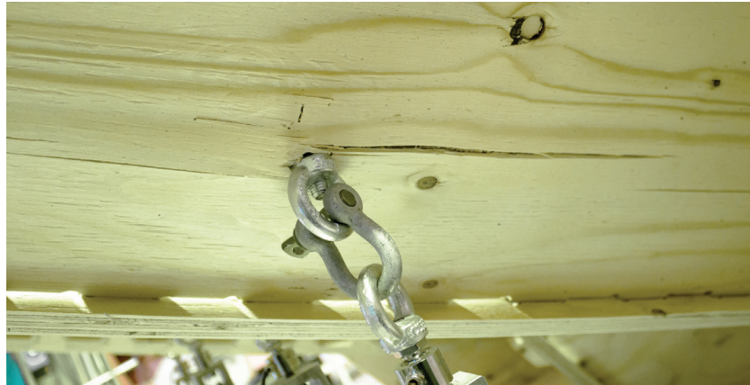
Figure 3.25 – MTSJ with closed slots, replicate 3. Failure along the middle of the loaded plate bottom face.
