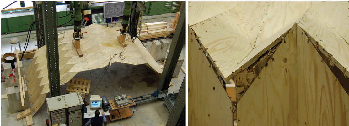
Figure 1.12 – Origami inspired plywood prototype testing and connection failure, H. Buri, Laboratory for Timber Constructions, EPFL, 2010.
